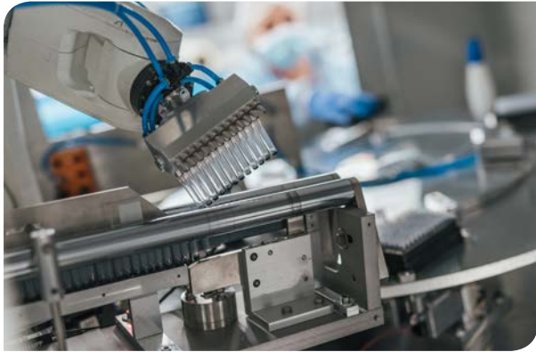
Automated Pick & Place for Tube Racking
