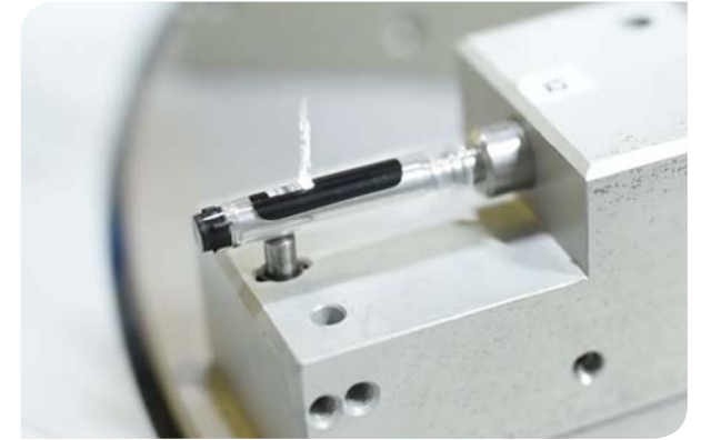
Single Tube Side Code Laser Etching
